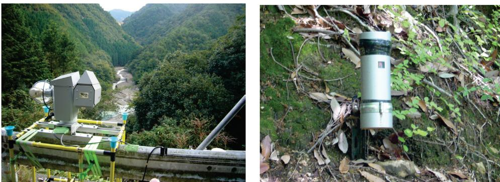
Photo.3 A debris-flow monitoring camera installed in the downstream of the Nagatono landslide dam (left) and a slope failure detection sensor (right)
