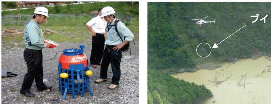
Photo.2 Photos of an aeriably-placable floating water stage gauge (APF gauge, left) and the APF gauge installed by a helicopter.
