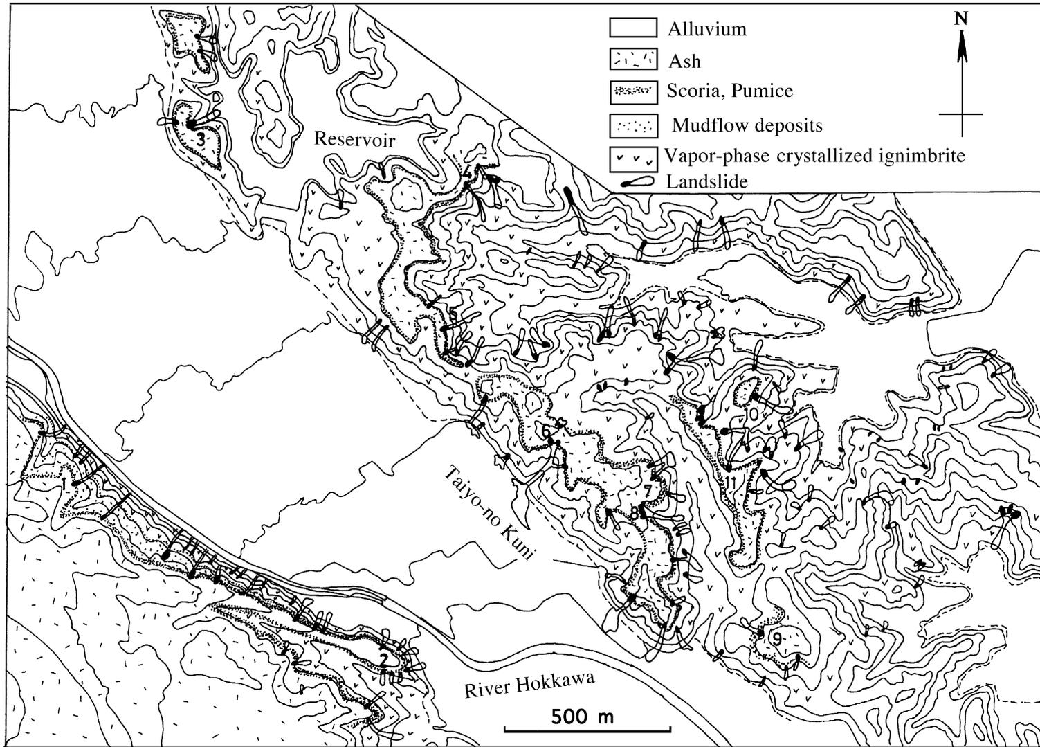
Fig. 3. Geologic map and landslide distribution around the Taiyo-no Kuni. Contour interval is 10 m.
