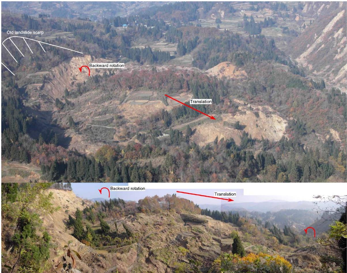
Fig. 10. Shiotani slide. Above: overview; below: side-looking view. The arrows indicate rotational and translational movements.
