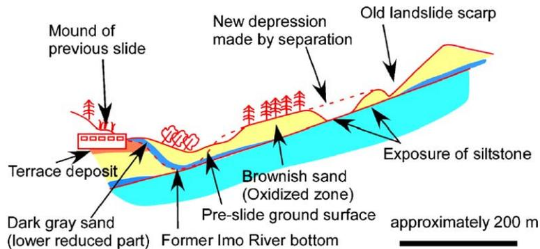
Fig. 5. Schematic cross-section of the Higashi-Takezawa slide.
